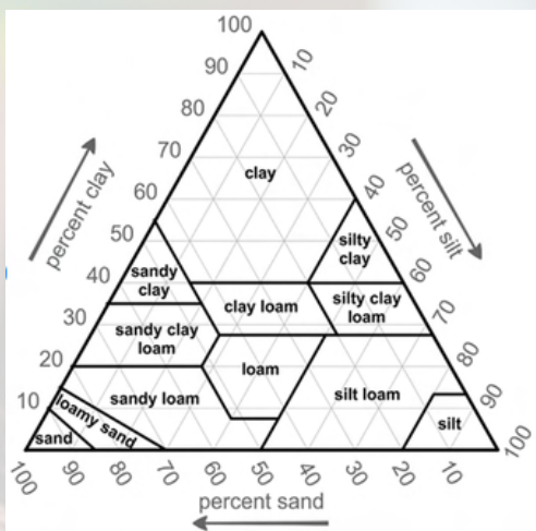
Figure 1: Soil texture type is based on a mixture of the relative percentages of clay, silt, and sand particles in a mass of soil. Source: USDA Soil Textural Triangle ( http://www.nrcs.usda.gov ).
